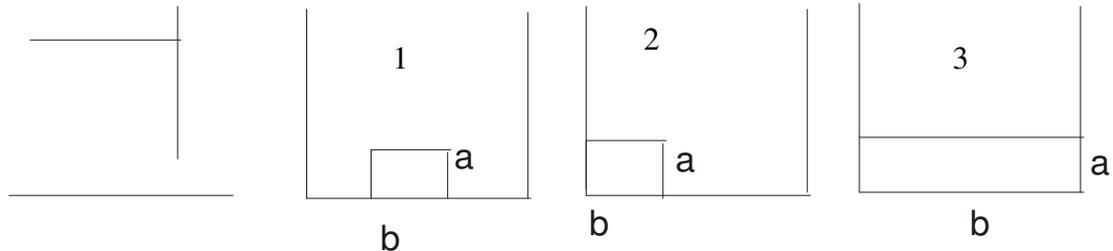
$$K_1 = \frac{b}{2(a+b)} \quad K_2 = \frac{a+b}{2(a+b)} \quad K_3 = \frac{2a+b}{2(a+b)}$$
