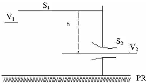
$$V_2 = C_v \sqrt{2gh + V_1^2}$$
